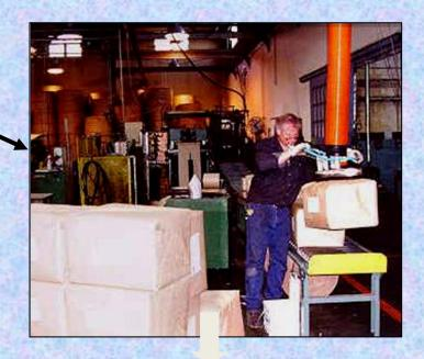
The example shown is palletizing using a vacuum lift at a paper mill that produces bundles of grocery bags. The vacuum lift costs around \$10,000, but in this case it increases productivity by allowing one employee to palletize on more than one line at a time without getting fatigued. It also allows rotation of all employees through this job, since physical capacity isn't a limiting factor.
