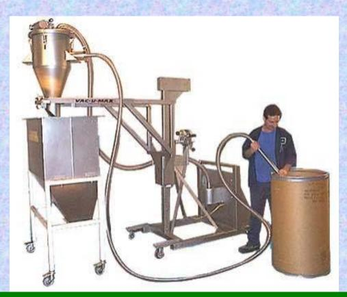
This example shows a mobile pneumatic conveyor that can be used to move powdered and granular materials from any type of container (bags, barrels, bins, totes, etc.) to a hopper or other part of a mixing system. The discharge (funnel shaped silver part at the top) is height adjustable.
