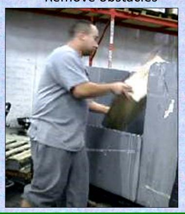
This shows lifting in and out of a tote with the side cut out. This can reduce the reach in many cases, although there will still be some awkward lifting. It's one of the cheapest solutions, since it just requires the time to cut out the side of the tote. Bins with flip-down sides are also available, so that as they fill up the sides can be flipped-up into place to hold the boxes in place.
