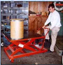
This is a relatively common device used in industry — a scissor-lift cart. The height of the cart is adjusted hydraulically, in this case with a foot pedal, although powered adjustment mechanisms are also available. These carts cost about \$1500.
