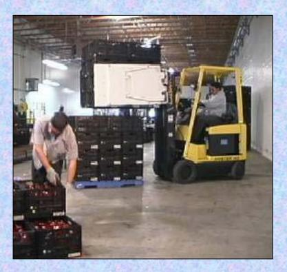
This example shows using a carton clamp on a forklift to split/combine two halves of a stack of bins, rather than un-stacking/stacking the top layers over shoulder height.
