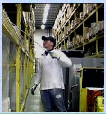
This example shows an order picking using an inexpensive (~\$15), metal hook, made in-house, to pull a box close to the edge of the shelf before lifting it. This works well for lighter items. Heavier items would need to be stored lower and slid closer using both hands.
