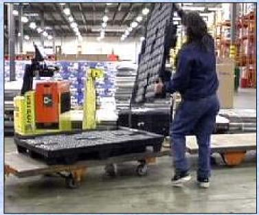
This example shows using lightweight plastic pallets, which weigh anywhere from 13 to 30 pounds for a standard 40" x 48" unit (the one in the picture is about 20 pounds). The traditional wooden 40" x 48" pallets weigh approximately 60 pounds.
